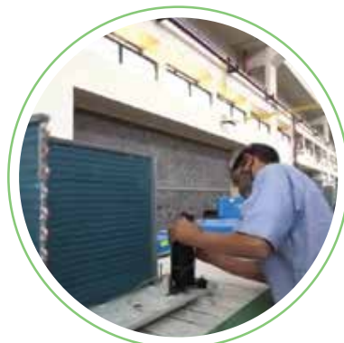
COMPRESSOR & CONDENSER FITMENT & BRAZING
