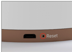
PT camera Reset button is at the bottom of the camera (next to adapter input)
